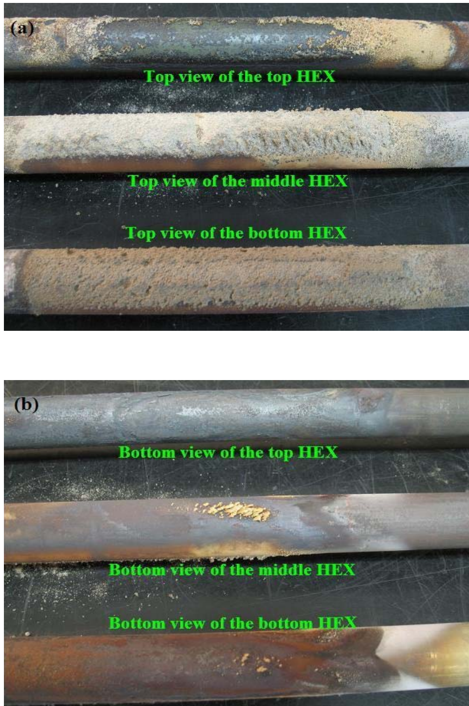
Figure 7.6. Ash depositions on HEXs for pure LAPCFB as a reburn fuel: (a) Top view of HEXs and (b) Bottom view of HEXs.
