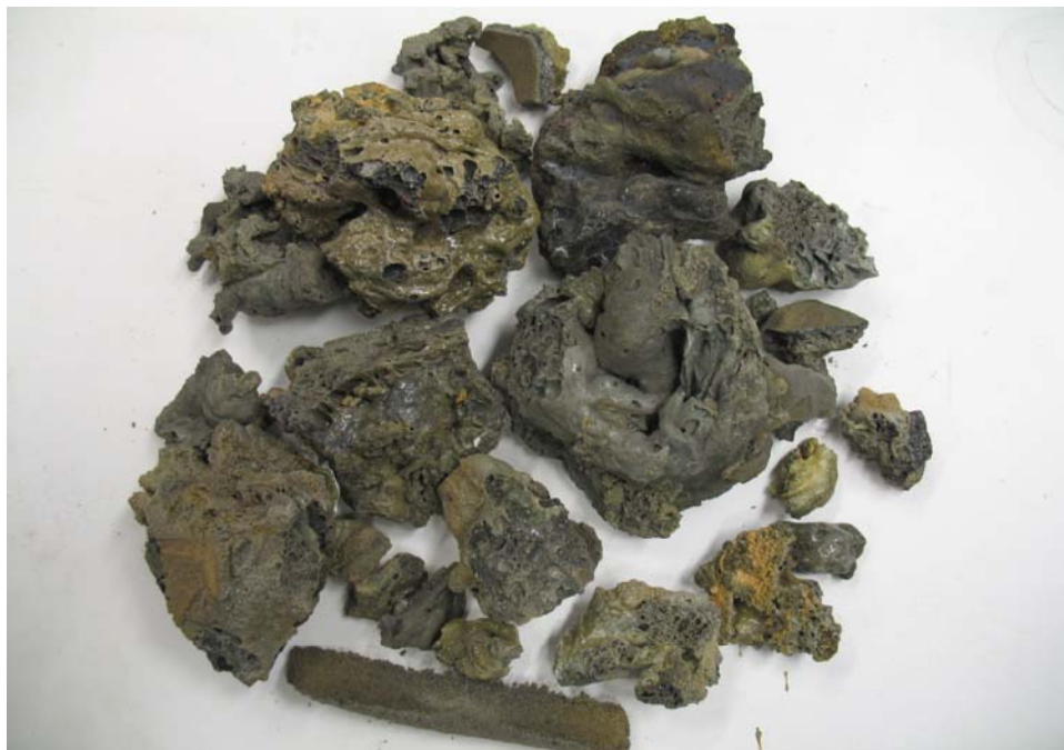
Figure 7.8. Molten behavior under the reburn burner with firing HAPCFB.
